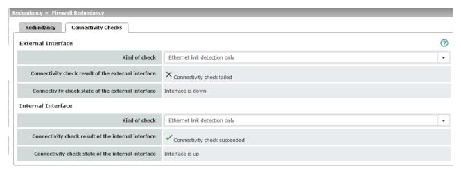
Targets can be configured for the internal and external interface in the connectivity check. It is important that these targets are actually connected to the specified interface. An ICMP echo reply cannot be received by an external interface when the corresponding target is connected to the internal interface (and vice versa). When the static routes are changed, the targets may easily not be checked properly.
